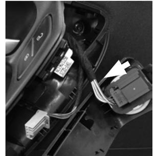
Loosen the screws which are located behind the grip dish and the torx screws at the door-panel (shown in the next illustration on the following side).
