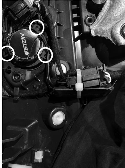
Remove the three fusion points of the tweeter with a sharp knife. Place the tweeter onto the pins of the speaker opening. Make sure that all the clips are properly fixed into place.
